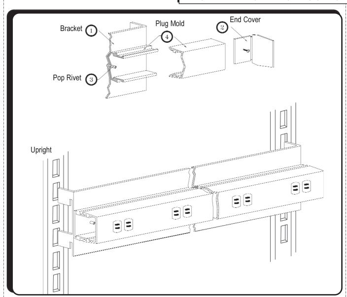
NOTE! The Plug Mold system installs into the uprights and is wired by a local electrician.
