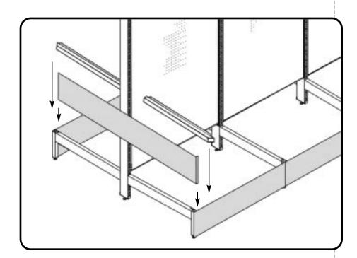
Side decks are tilted up, then down to lock brackets into uprights. Tabs on uprights should locate to the outside of the base decks.
