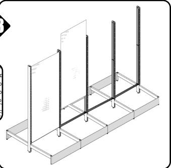
If upright extensions are used, install them into the tops of the uprights. Install back panel extensions once upright extensions are secured.
