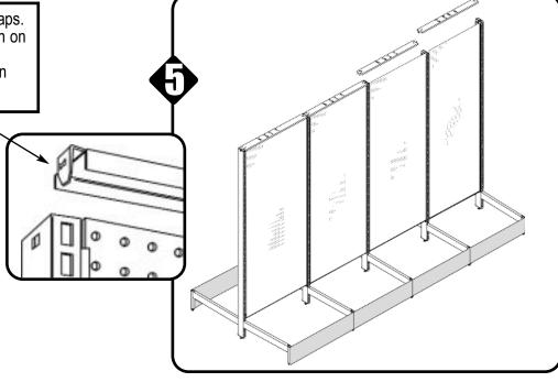
Next, adjust uprights so that the entire run is in alignment with the chalk line. NOTE: Recheck chalk line carefully for accuracy. Madix is not responsible for damages resulting from moving an assembled fixture. Plumb by using a level on the face of each upright while adjusting the outer leveling legs. The center leveling leg of all uprights should be run out and left at a clearance of approximately 3/16", or the thickness of the leveler wrench.
