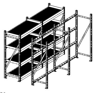
STEP 2 SETUP SECOND RUN WITH ONLY THE BEAMS ADJACENT TO THE FIRST RUN INSTALLED ON THE FRAMES
